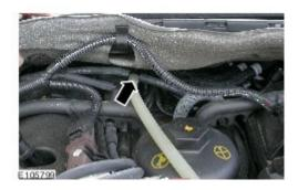
If there is no leak at the port deactivation valves, carry out steps 7 and 8 and return the vehicle to customer. If a leak is detected at the port deactivations valve(s), carry on from step 8.
